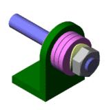
Friction disc: a waved spring is clamped on the shaft against a stop by means of a nut or a retaining bracket. The torque is generated by the tension of the wave spring.
