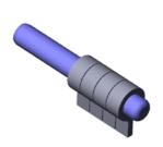
"Question Mark" spring band: a steel band with approximately the shape of a question mark is mounted on the shaft. One end of the steel band is firmly connected to the stationary part of the hinge, the other to the moving part of the hinge. The torque is generated by pressure from the inside of the steel band on the outside diameter of the shaft.
