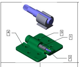
Clip technology: the patented clip technology transmits the torque through several clips (1), which are pressed onto the shaft (2) One part of the hinge (3) is connected to the ends of the shaft, the other part (4) is attached to the "foot" of the clips. When rotating around the axis, a consistent static and dynamic frictional torque is generated between the axis and the clips.
