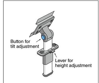
The tilt adjustment unlocks while the button is pushed.
