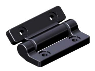
Reell's MH15 position hinge utilizes the TI-240 in its overmolded design. The TI-240 is centered in the mold using the shaft chamfers, which completely covers the shaft ends and has no visible holes in the plastic over the knurled portion of the shaft.
