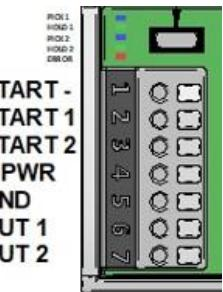
Terminals 1 (Negative), 2 (Start1) and 3 (Start2) are the opto-isolated control inputs. The input circuit is as shown below, applying 5v-30v to this will switch the circuit 'ON'. Higher control voltage may be used if appropriate serial resistor is inserted to limit the input current to 6mA.
