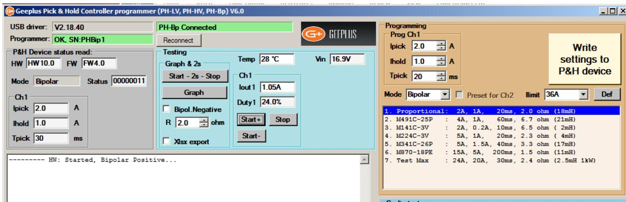
In Bipolar mode, the polarity of excitation with the ‘Start – 2s – Stop’ function or the ‘Graph’ function is determined by the checkbox ‘Bipol.Negative’. Checking or unchecking this box reverses the excitation direction of subsequent cycles.
