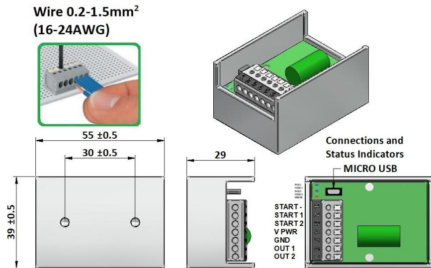
Standard module configuration is mounted in a die-cast box and potted (encapsulated) with resin.
