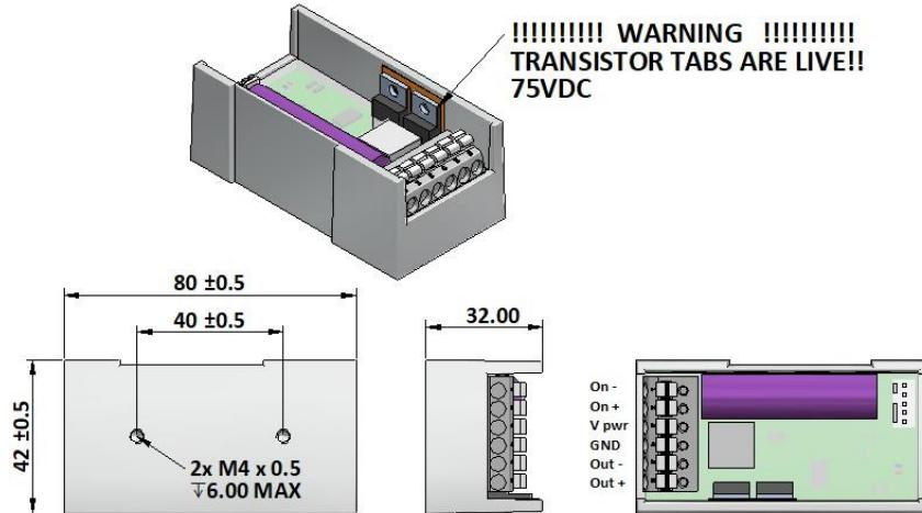
Standard module configuration is mounted in a die-cast box and potted (encapsulated) with resin.
