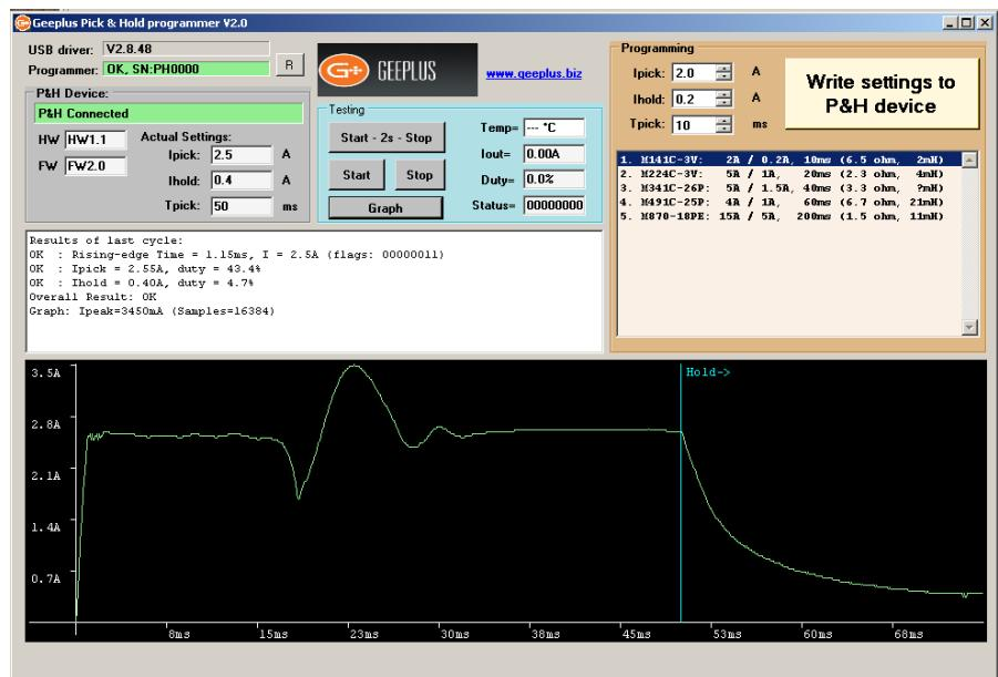
The ‘Graph’ display shows the current vs time for an interval of 1.5x the chosen ‘Pick’ time. The graphical display allows the user to visualise the following parameters:
