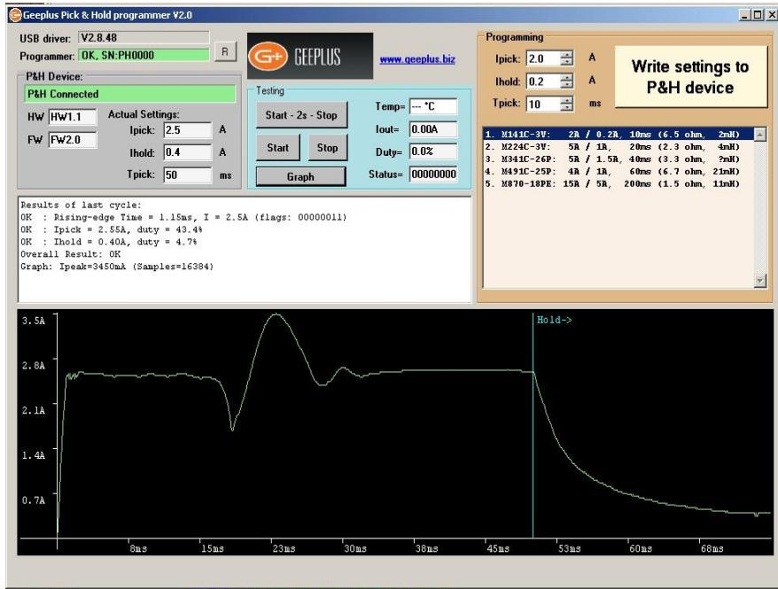
When connected to a PC/Laptop a clear graphical display of the excitation current waveform can be observed. This helps users select an appropriately sized solenoid for the application and optimise the excitation current conditions to achieve the required force or speed with minimum power consumption and heat dissipation.
