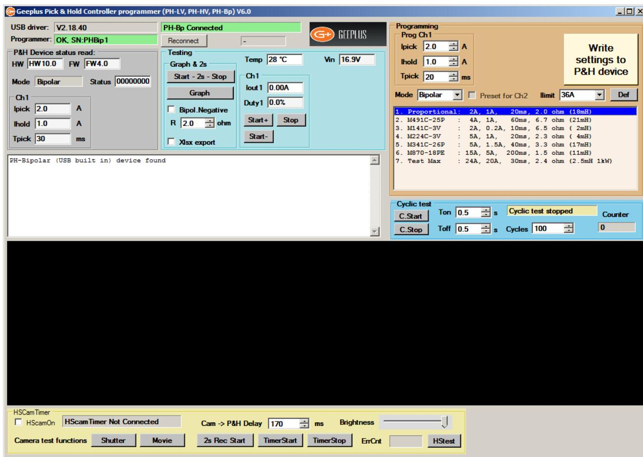
Note: the programmer reads the actual settings from the module, and it will appear with different controls regarding the actual Mode (above showing Bipolar).
