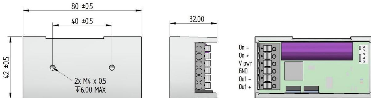
The standard module configuration is mounted in a die-cast box and potted (encapsulated) with resin.
