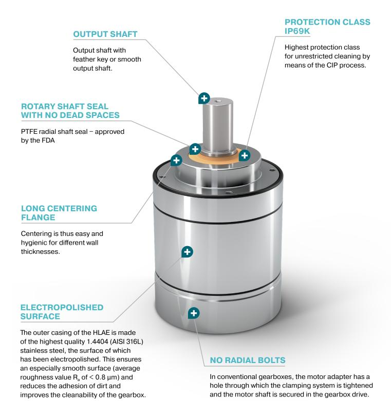
The HLAE does not need this hole. The surface remains absolutely round, even in the area of the motor adapter, so that no biofilm residue can adhere.
