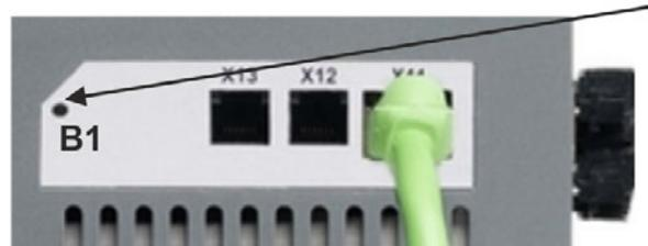
3. When the display blinks with the set rotary switch setting stop pushing B1 and wait until the blinking stops. During that time the parameter FBUS.PARAM01 is set to the new value and all parameters are stored to the non volatile memory. The new setting will be taken with the next power-up of the drive.
