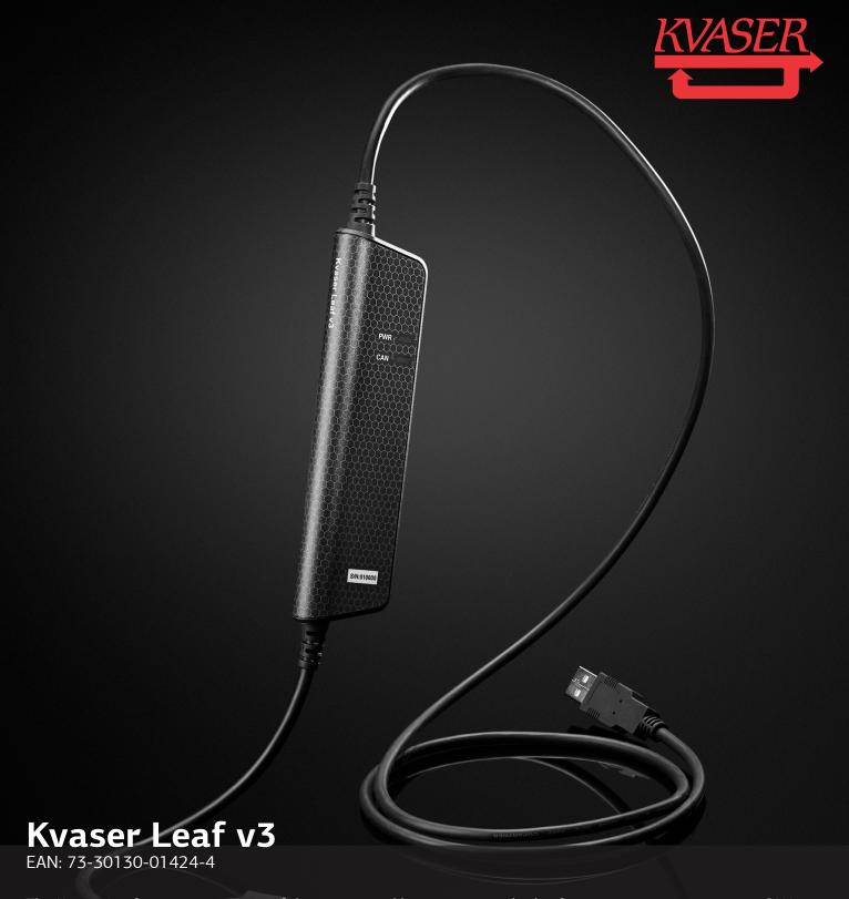
The Kvaser Leaf v3 represents one of the easiest and lowest-cost methods of connecting a computer to a CAN bus network in order to monitor and transmit CAN and CAN FD data. With its standard USB type "A" connector and 9-pin D-SUB connector, the Leaf v3's sleek, ergonomically designed housing is both robust enough for every-day use and small and flexible enough to be used in space-constrained applications.
