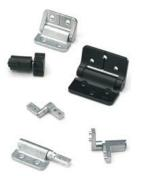
Constant torque hinges (also known as friction hinges, frictional hinges, positioning hinges) are purely mechanical components that serve to automatically hold an object that has been brought into any angular position there. Typical applications include laptop screens, monitors in industrial applications, special cases, office equipment, equipment protection devices, access hatches, etc.
