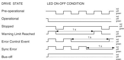
Note: Red & green led on-times do not overlap. LED color may be red, green, off, or flashing of either color.
