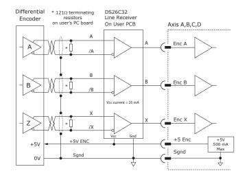
This graphic shows both encoder and line-receiver powered from the ME4 +5V output. If four encoders are connected like this, and assuming 25 mA for each line-receiver, then the available +5V power for each encoder would be 100 mA.
