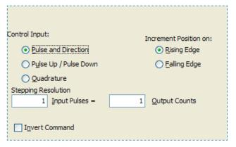
This screen shows the configuration screen for Pulse & Direction. CU/CD and Quad A/B encoder are selectable on this screen, too.
