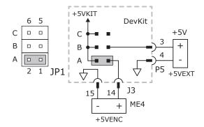
IMPORTANT: ONLY ONE SHORTING PLUG CAN BE USED ON JP1-A or JP1-B POSITIONS USE OF MORE THAN ONE PLUG WILL DAMAGE 5V POWER SUPPLIES IN THE ME4
