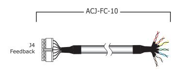
This cable plugs into drive J4 and consists of seven twisted-pairs of AWG 24 wire. Each pair has a black and colored conductor. The chart above shows twisted-pairs in the rows. E.g. one pair goes to pins 1&8, another pair to pins 2&9, etc. Cable termination is flying leads for connection to customer motor feedback encoder.
