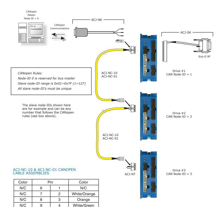
These cables connect to amplifier J1 and have 3 conductors of AWG 24 wire that are terminated in contacts that can then be inserted into pins  $7\sim9$  of another ACJ-NC-10 to "daisy chain" the CAN signals to multiple amplifiers.
