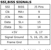
Note: Single (outer) shields should be connected at both ends (motor and drive frame grounds). Inner shields should only be connected to Signal Ground on the drive.
