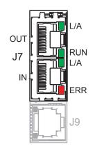
J7: EtherCAT PORTS RJ-45 receptacles, 8 position, 4 contact
