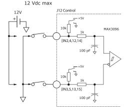
PLC outputs are frequently current-sourcing from 24V for driving grounded loads. PC based digital controllers commonly use NPN or current-sinking outputs. Set the Xenus inputs to pull-down to ground for current-sourcing connections, and to pull-up to 5V for current-sinking connections.
