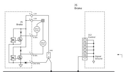
Earthing connections for power supplies should be as close as possible to elimimate potential differences between power supply 0V terminals.
