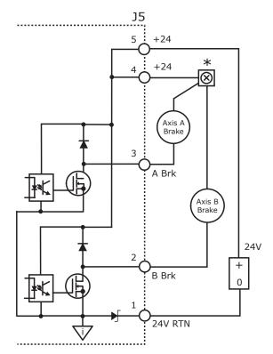
★ There should be only one conductor in each position of the J5 connector. If brakes are to be wired directly to J5 for their 24V power, use a double wire ferrule for J5-4. Information for ferrules can be found on page 30.
