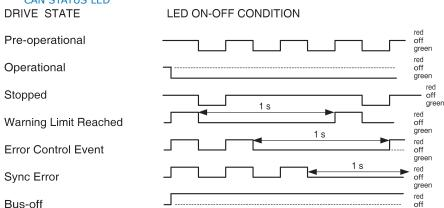
Note: Red & green led on-times do not overlap. LED color may be red, green, off, or flashing of either color.
