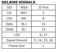
Note: Single (outer) shields should be connected at both ends (motor and drive frame grounds). Inner shields should only be connected to Signal Ground on the drive.
