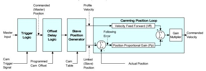
Note that during camming, profile velocity, acceleration, deceleration, and Aff have no effect. The only limiting variables are the current limits and the velocity limit in the velocity loop.
