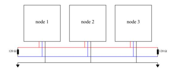
Messages are transmitted on the CAN bus as a series of bits. 0 bits (called dominate bits in CAN terminology) are signaled by applying a differential voltage between the CAN\_H and CAN\_L bus lines. 1 bits (called recessive bits in CAN) are signaled by not driving the bus and allowing the terminating resistors to reduce the differential voltage to zero.
