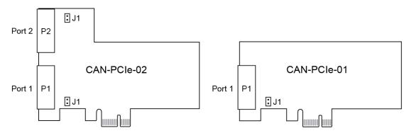
The card uses a single lane PCI express connector to interface with the host computer. The card can be installed in any PCI express slot on the host PC, both single lane slots and multi-lane slots will work equally well. To install the card in the host PC, power down the PC and insert the card into any free PCI express slot. We recommend that a screw be used to secure the bracket to the host chassis.
