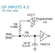
\* [IN5] connects to J2 for motor overtemp switch
